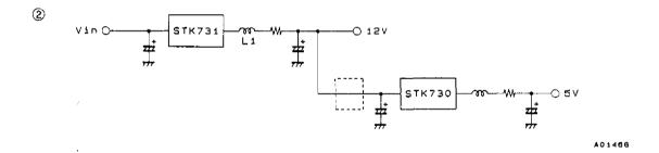
Note: It is possible for STK730 input ripple currents to cause L1 to vibrate audibly and adversely influence the 12 V system. If such problems occur, an inductor can be inserted at the point marked with dotted lines in the figure above to form an LC filter.
