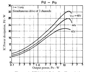
Figure 1. STK4412 Pd – Po ( $R_L = 8\Omega$ )
