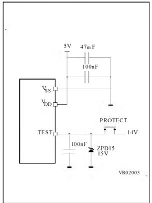
Note: ZPD15 is used for overvoltage protection
