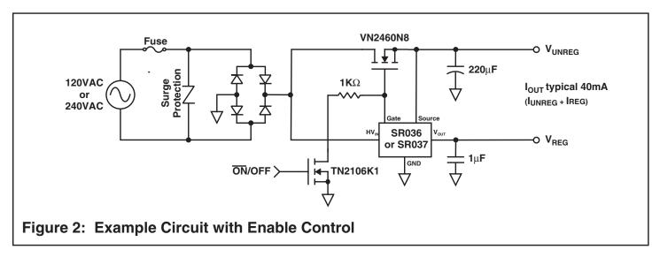
Figure 2 is an example circuit using the SR036 or SR037 along with a Supertex VN2460N8 MOSFET to generate an unregulated voltage of approximately 18V and a regulated voltage of 3.3V for the SR036 or 5.0V for the SR037. The combined total
