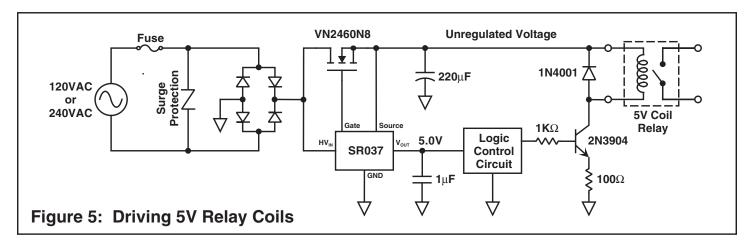
The circuit shown in Figure 5 uses the SR037 to supply a regulated 5.0V for the logic control circuitry while the unregulated voltage is used to drive a 5.0V coil relay. To overcome the voltage variation of the unregulated line, a bipolar transistor is
