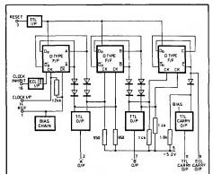
Fig.2 SP8735/6 logic diagram
