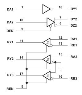
While the SN75LBC773 is powered off ( $V_{CC}$  and  $V_{EE} = 0$ ), the outputs are in a high-impedance state. A logic high on the driver enable (DEN) or logic low on the receive enable (REN) terminals places the outputs of the differential driver and receivers, respectively, into a high-impedance state. All drivers and receivers have fail-safe mechanisms that ensure a high output state when the inputs are left open.
