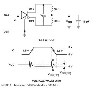
Figure 3. Differential Driver Common-Mode Output Voltage Test Circuit
