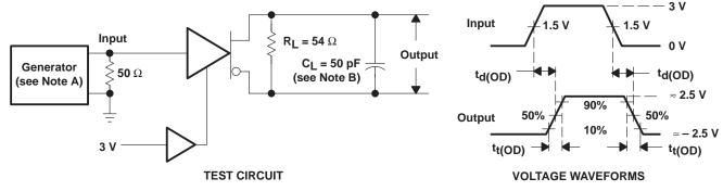
NOTES: A. The input pulse is supplied by a generator having the following characteristics: PRR  $\leq$  1 MHz, duty cycle = 50%, t<sub>r</sub>  $\leq$  5 ns, t<sub>f</sub>  $\leq$  5 ns, Z<sub>O</sub> = 50  $\Omega$ .
