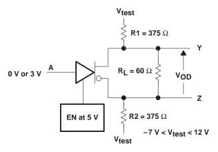
Figure 2. Driver V<sub>OD</sub> Test Circuit
