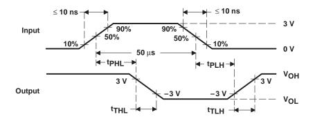
NOTES: A. The pulse generator has the following characteristics: duty cycle  $\leq$  50%,  $Z_O\approx$  50  $\Omega$
