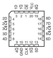
OE does not affect the internal operations of the flip-flops. Old data can be retained or new data can be entered while the outputs are off.
