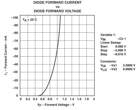
Figure 1. Current Versus Voltage for the SN74F1056
