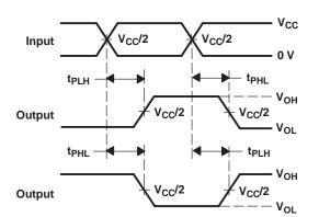
**VOLTAGE WAVEFORMS** SETUP AND HOLD TIMES  $V_{CC}$ Output V<sub>CC</sub>/2 V<sub>CC</sub>/2 Control 0 V Output Waveform 1 Vcc S1 at 2  $\times$   $V_{CC}$ V<sub>CC</sub>/2 (see Note B)  $V_{OL}$ Output  $V_{OH}$ Waveform 2 **V<sub>OH</sub> - V**<sub>\(\)</sub> V<sub>CC</sub>/2 S1 at GND ≈0 V (see Note B)
