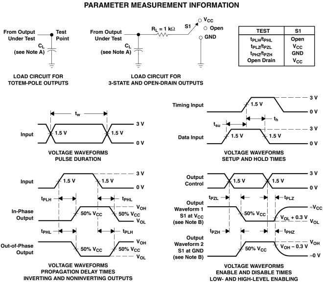
NOTES: A. C<sub>L</sub> includes probe and jig capacitance.
