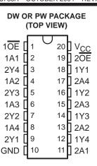
To ensure the high-impedance state during power up or power down,  $\overline{OE}$  should be tied to V<sub>CC</sub> through a pullup resistor; the minimum value of the resistor is determined by the current-sinking capability of the driver.
