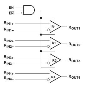
The intended application of this device and signaling technique is for point-to-point baseband data transmission over controlled impedance media of approximately 100  $\Omega$ . The transmission media may be printed-circuit board traces, backplanes, or cables. The ultimate rate and distance of data transfer is dependent upon the attenuation characteristics of the media, the noise coupling to the environment, and other system characteristics.
