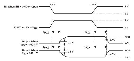
Figure 4. Receiver 3-State Delay Waveforms
