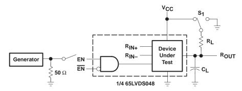
$C_L$  Includes Load and Test Jig Capacitance.  $S_1 = V_{CC}$  for  $t_{PZL}$  and  $t_{PLZ}$  Measurements.
