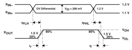
Figure 2. Receiver Propagation Delay and Transition Time Waveforms
