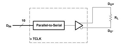
$V_{OD}$  = (D<sub>O</sub>+) - (D<sub>O</sub>-) Differential Output Signal Is Shown as (D<sub>O</sub>+) - (D<sub>O</sub>-)
