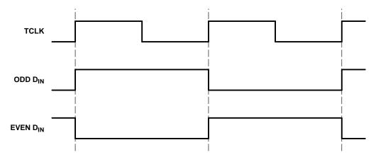
Figure 2. Worst-Case Serializer  $\rm I_{\rm CC}$  Test Pattern
