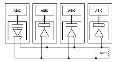
Figure 21. Multidrop Configuration
