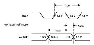
Figure 8. Serializer Setup/Hold Times
