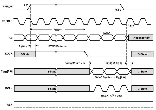
Figure 16. Deserializer PLL Lock Times and PWRDN 3-State Delays
