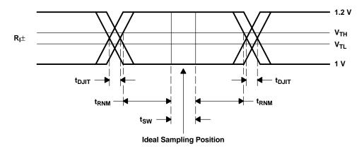
t<sub>SW</sub>: Setup and Hold Time (Internal Data Sampling Window)
