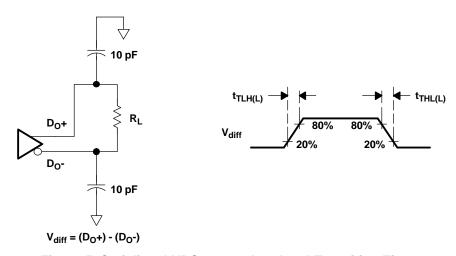
Figure 5. Serializer LVDS Output Load and Transition Times
