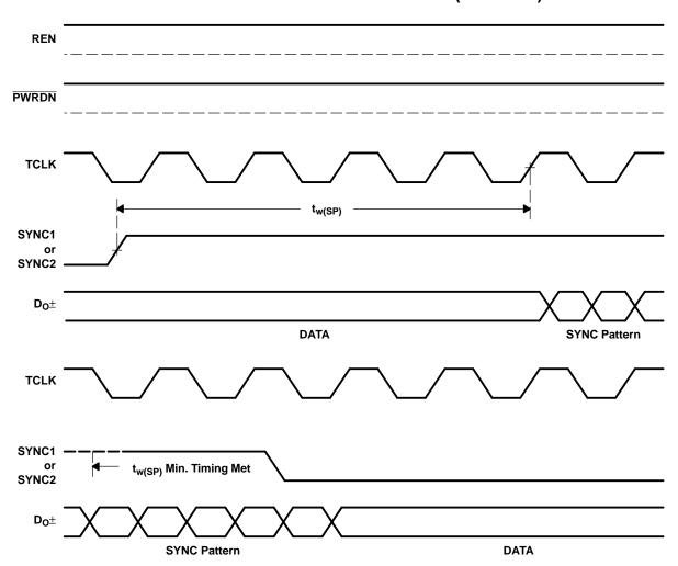
Figure 11. SYNC Timing Delays
