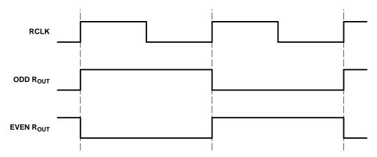
Figure 4. Worst-Case Deserializer  $I_{CC}$  Test Pattern
