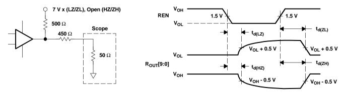
Figure 15. Deserializer High-Impedance-State Test Circuit and Timing
