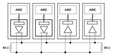
Figure 22. Multiple Serializers and Deserializers on the Same Differential Bus
