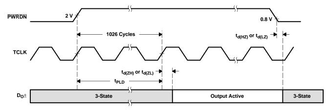
Figure 10. Serializer PLL Lock Time and PWRDN High-Impedance-State Delays
