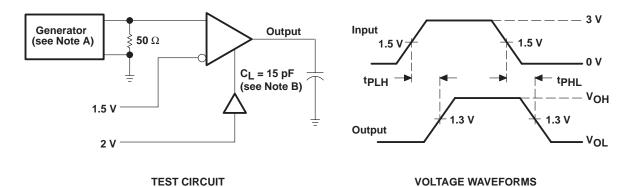
NOTES: A. The input pulse is supplied by a generator having the following characteristics: PRR  $\leq$  1 MHz, duty cycle  $\leq$  50%, Z<sub>O</sub> = 50  $\Omega$ ,  $t_f \leq$  6 ns,  $t_f \leq$  6 ns.
