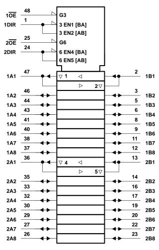
logic diagram (positive logic)
