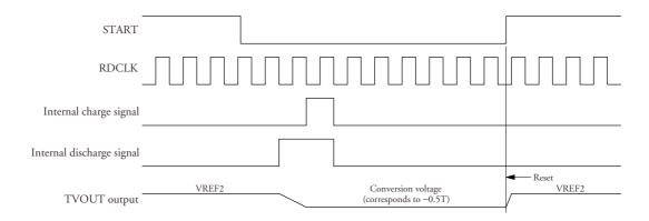
Figure 3. Converter coefficient measurement mode timing (POLAR = LOW)
