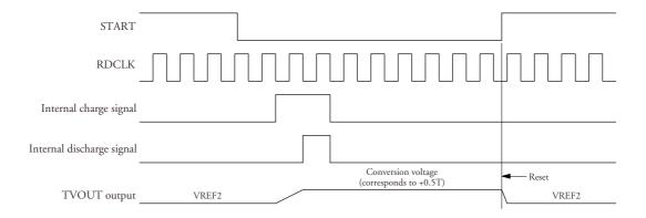
Figure 4. Converter coefficient measurement mode timing (POLAR = HIGH)
