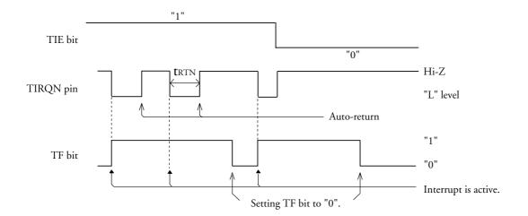
The auto-return time ( $t_{RTN}$ ), shown in the following figure and table, is determined by the source clock frequency set by register 8 in bank 2 bits TD0 and TD1.
