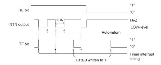
The auto-return time  $(t_{\text{RTN}})$  is determined by the source clock frequency set by register address C as shown in the following table.
