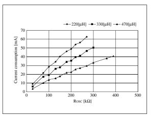
Figure 22. R<sub>OSC</sub> – Current consumption
