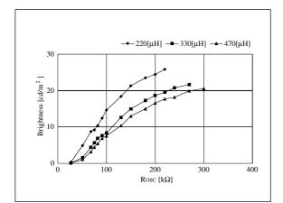
Figure 30. R<sub>OSC</sub> – Brightness
