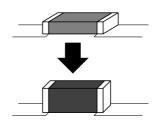
Furthermore, if the chip capacitor is mounted laying on its side, then the contact area with the PCB is minimized which will also help reduce noise.
