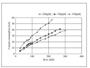
Figure 31. R<sub>OSC</sub> – Current consumption
