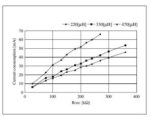
Figure 37. R<sub>OSC</sub> – Current consumption
