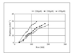
Figure 42. R<sub>OSC</sub> – Brightness
