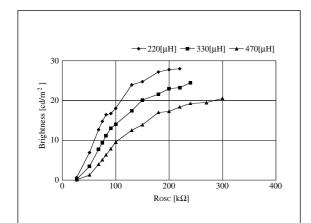
Figure 18. R<sub>OSC</sub> – Brightness
