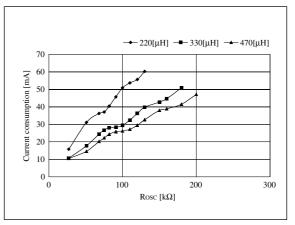
Figure 43.  $R_{OSC}$  – Current consumption
