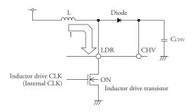
Figure 6. Boost circuit (transistor ON)
