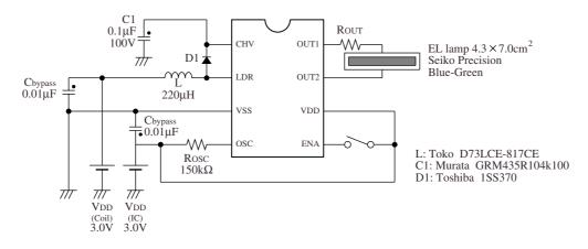
Figure 9. Output waveform adjustment circuit
