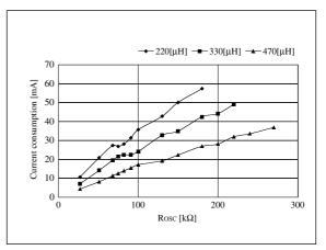
Figure 28. R<sub>OSC</sub> – Current consumption
