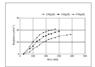
Figure 21. R<sub>OSC</sub> – Brightness
