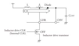
Figure 7. Boost circuit (transistor OFF)
