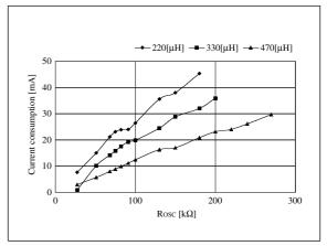
Figure 16. R<sub>OSC</sub> – Current consumption
