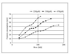
Figure 40. R<sub>OSC</sub> – Current consumption
