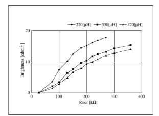
Figure 36. R<sub>OSC</sub> – Brightness
