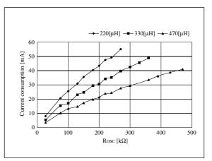
Figure 25.  $R_{OSC}$  – Current consumption
