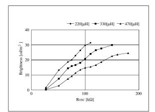
Figure 39. R<sub>OSC</sub> – Brightness
