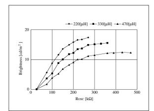
Figure 24. R<sub>OSC</sub> – Brightness
