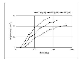
Figure 27. R<sub>OSC</sub> – Brightness
