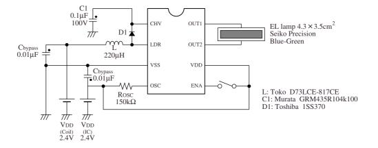
Figure 14. Application circuit
