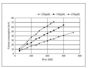
Figure 34. R<sub>OSC</sub> – Current consumption
