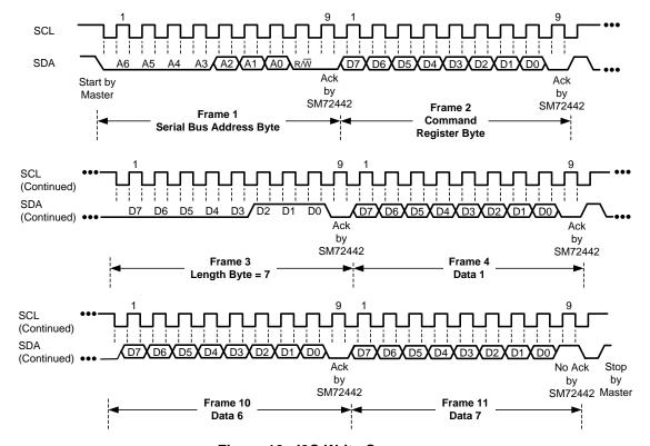
Figure 12. I2C Write Sequence
