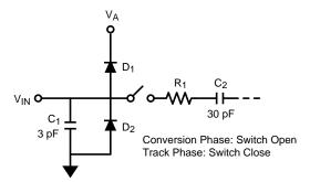
Figure 9. Equivalent Input Circuit
