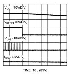
Figure 8. Forced Reset Condition
