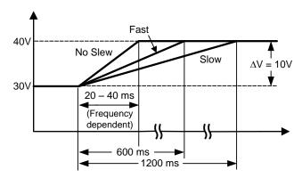
Figure 6. Slew Rate Limitation Circuit
