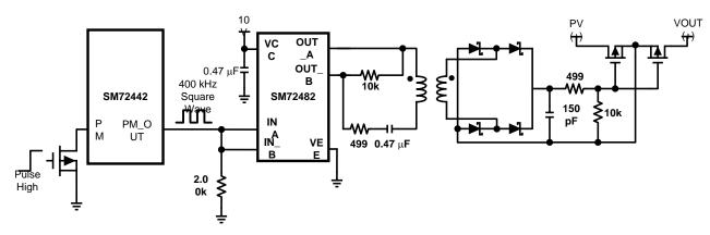
Figure 7. Sample Application for Panel Mode Operation
