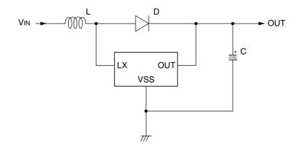
Coil (L) : 330 $\mu$ H Diode (D) : MA721 (Matsushita Schottky diode) Capacitor (C<sub>L</sub>) : 22 $\mu$ F tantalum
