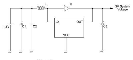
Coil (L) : 330µH Schottky Diode (D) Capacitor (C1) : 22µF tantalum Capacitor (C2) : 0.22µF ceramic Capacitor (C3) : 22µF tantalum
