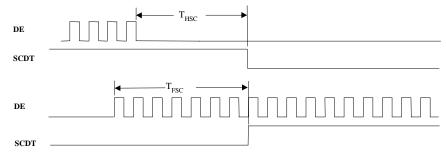
Figure 6. SCDT Timing from DE Inactive/Active
