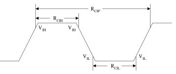
Figure 2. Receiver Clock Cycle/High/Low Times
