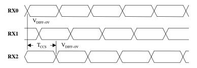
Figure 3. Channel-to-Channel Skew Timing
