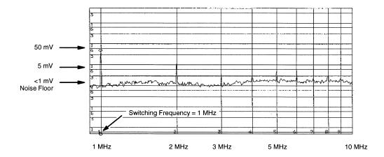
FIGURE 9. Higher resolution of noise spectrum
