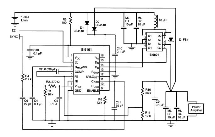
FIGURE 1. Si9161 Boost Converter
