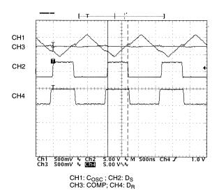
FIGURE 2. Gate Drive Timing Diagrams
