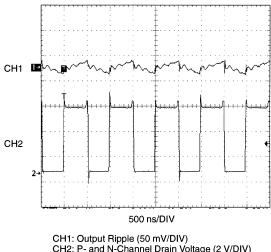
CH2: P- and N-Channel Drain Voltage (2 V/DIV)
