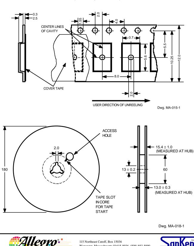
**Tape and Reel Dimensions in Millimeters** (controlling dimensions)
