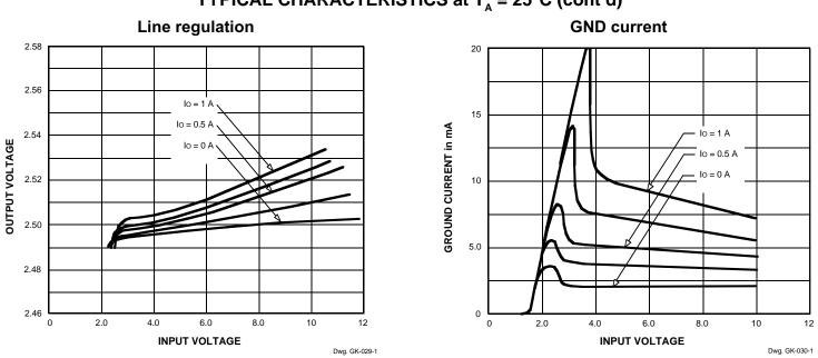
TYPICAL CHARACTERISTICS at  $T_A = 25^{\circ}C$  (cont'd)
