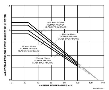
Leads 7 and 8 are soldered to the copper area and provide heat sinking of the pass transistor.
