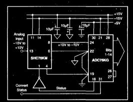
FIGURE 2. A 20kHz A/D Conversion System (14-bit accurate).
