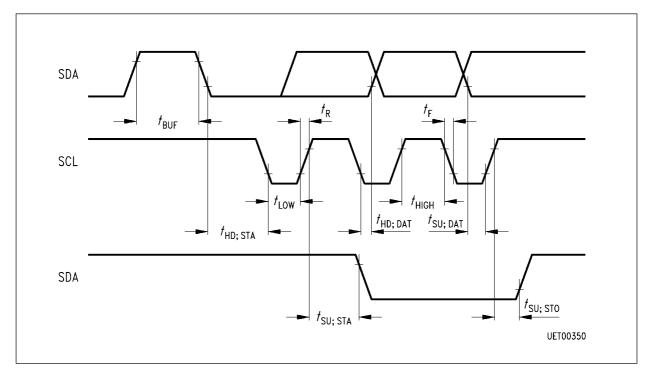
Figure 2 Timing Conditions for the  ${\bf I}^2{\bf C}$  Bus (high-speed mode)
