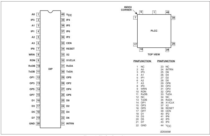
Figure 1. Pin Configurations
