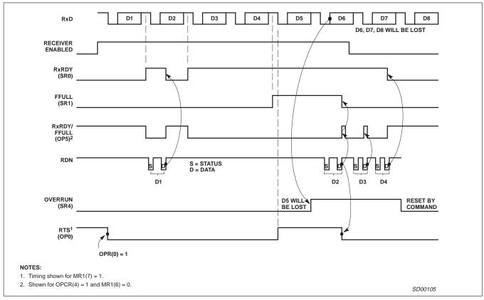
Figure 11. Receiver Timing
