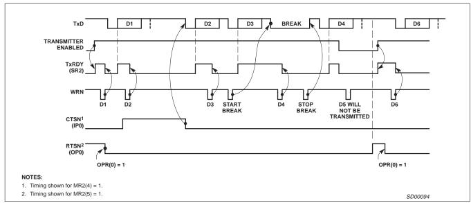
Figure 10. Transmitter Timing
