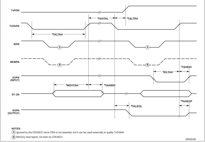
Figure 14. DMA-Transmit Single Address Mode
