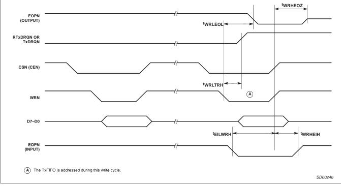
Figure 12. Transmit Dual Address DMA Timing
