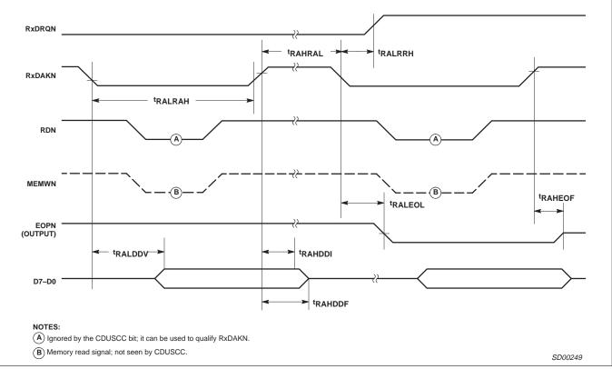
Figure 15. DMA-Receive Single Address Mode
