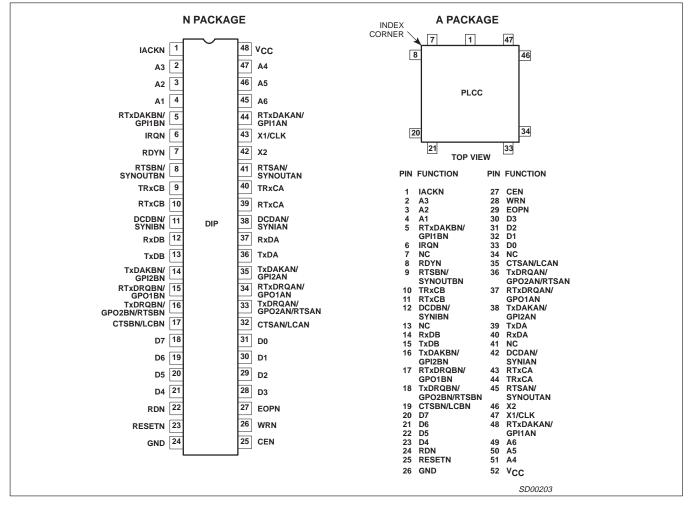
Figure 1. Pin Configurations
