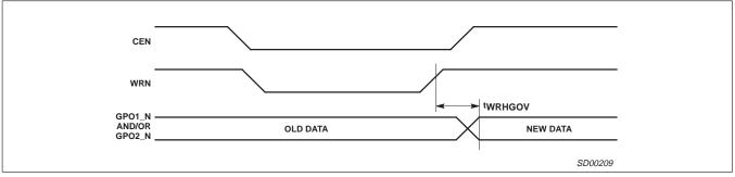
Figure 7. Output Port Timing
