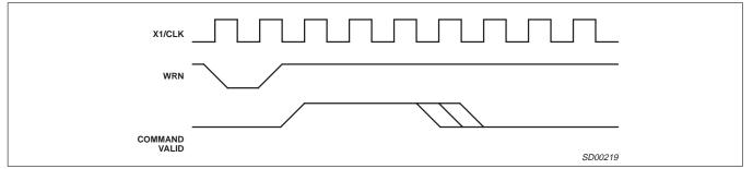
Figure 17. Command Timing
