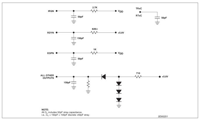
Figure 20. Test Conditions for Outputs
