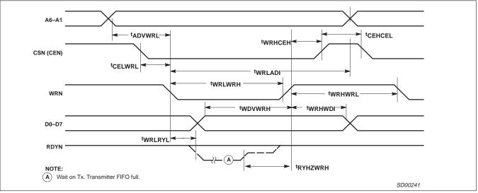
Figure 5. Write Cycle<sup>12</sup>
