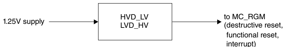
Figure 5-2. Logic scheme of the core voltage detectors
