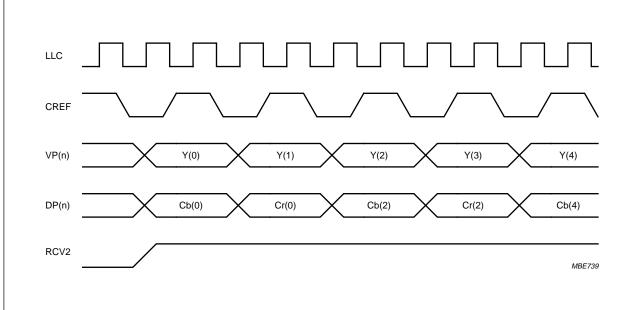
The data demultiplexing phase is coupled to the internal horizontal phase.
