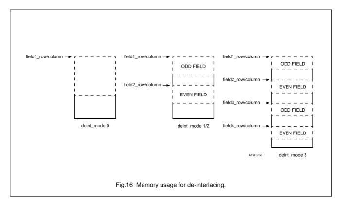
The memory interface addresses alternately the two banks of the SDRAM or SGRAM devices. So the memory needs for the field stores must be calculated from the following formula:
