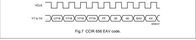
The CCIR 656 code byte contains vertical and horizontal blanking as well as odd and even field information, the protection bits P3 to P0 are ignored.
