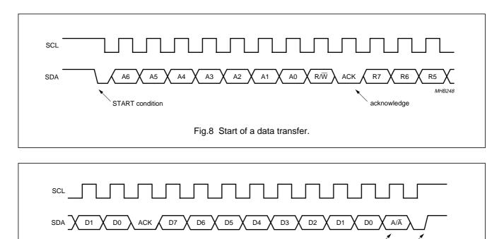
Fig.9 End of a data transfer.
