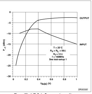
Figure 28. 1dB Gain Compression vs V<sub>AGC</sub>
