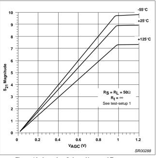
Figure 16. Insertion Gain vs V<sub>AGC</sub> and Temperature
