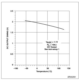
Figure 22. DC Output Swing vs Temperature
