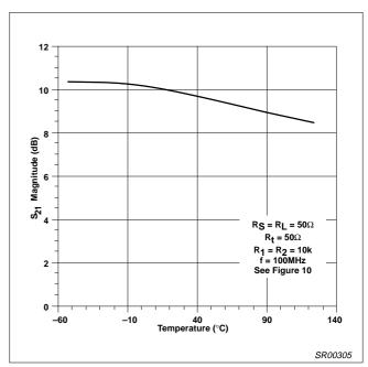
Figure 33. Fixed Gain vs Temperature
