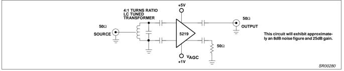
Figure 8. Narrowband Gain Optimization
