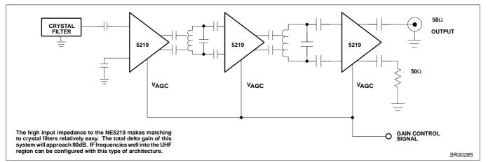
Figure 13. Receiver AGC IF Gain
