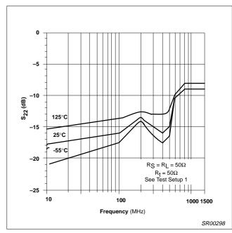
Figure 26. Output Return Loss vs Frequency
