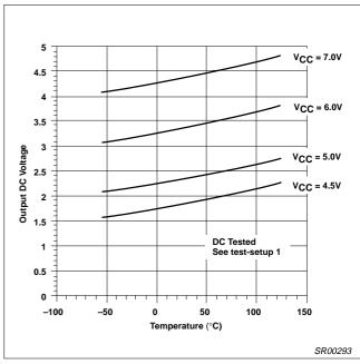
Figure 21. Output Bias Voltage vs Temperature and  $V_{\mbox{CC}}$
