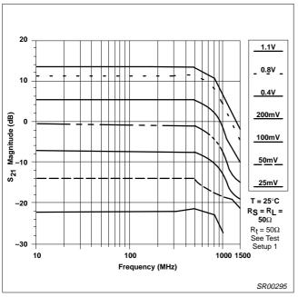
Figure 23. Insertion Gain vs Frequency and  $V_{\mbox{\scriptsize AGC}}$
