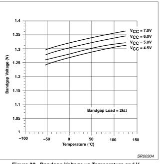
Figure 32. Bandgap Voltage vs Temperature and  $V_{\text{CC}}$
