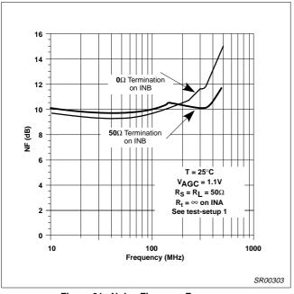
Figure 31. Noise Figure vs Frequency
