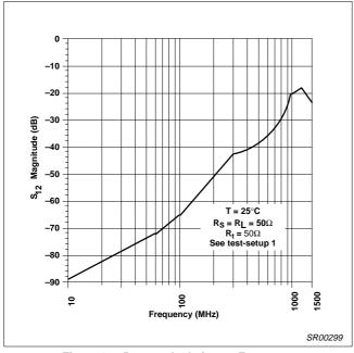
Figure 27. Reverse Isolation vs Frequency
