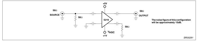
Figure 9. Simple Amplifier Configuration
