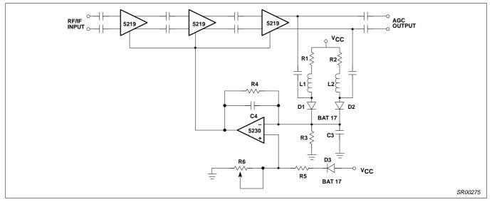
Figure 3. AGC Configuration Using Cascaded NE5219s
