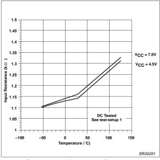
Figure 19. Input Resistance vs Temperature
