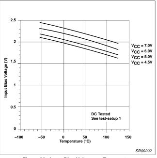
Figure 20. Input Bias Voltage vs Temperature
