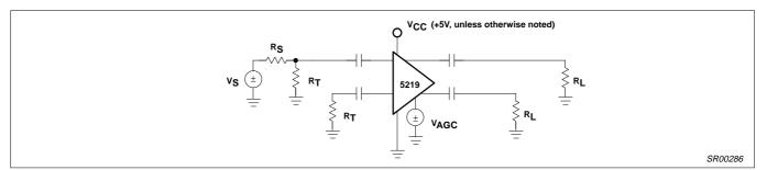
Figure 14. Test Set-up 1 (Used for all Graphs)
