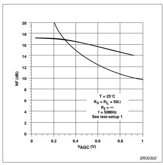
Figure 30. Noise Figure vs V<sub>AGC</sub>
