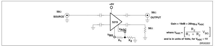
Figure 11. User-Programmable Fixed Gain Block
