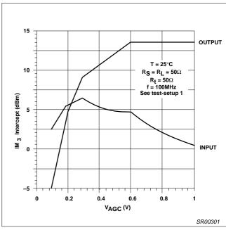
Figure 29. Third-Order Intermodulation Intercept vs V<sub>AGC</sub>
