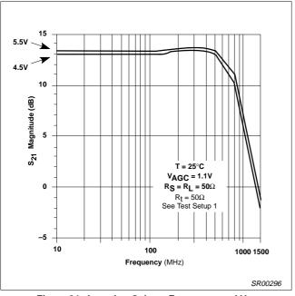
Figure 24. Insertion Gain vs Frequency and V<sub>CC</sub>
