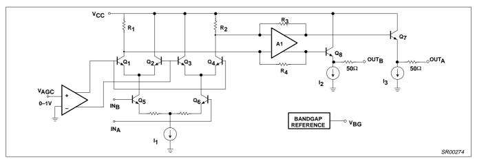
Figure 2. Equivalent Schematic of VGA
