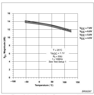
Figure 25. Insertion Gain vs Temperature and  $V_{\mbox{\footnotesize{CC}}}$
