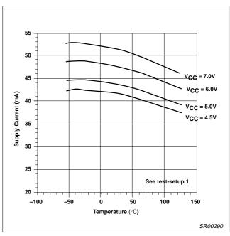
Figure 18. Supply Current vs Temperature and V<sub>CC</sub>
