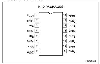
Figure 1. Pin Configuration
