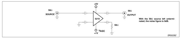
Figure 10. Unterminated Configuration
