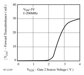
Figure 4. Forward Transadmittance vs. Gate 2 Source Voltage
