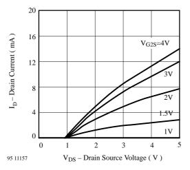
Figure 2. Drain Current vs. Drain Source Voltage
