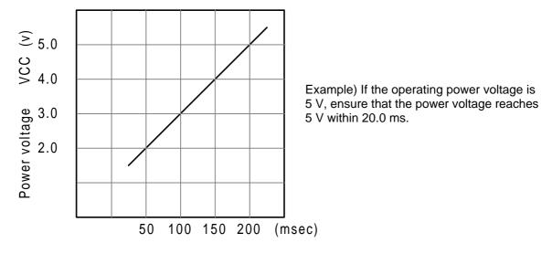
Fig. 2 Maximum power-voltage activation time
