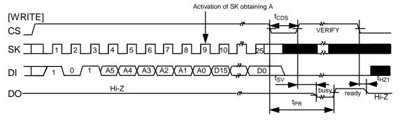
Case in which, during a command entry, CS is changed from H to L with a timing that differs by a predetermined minimum number of clocks.
