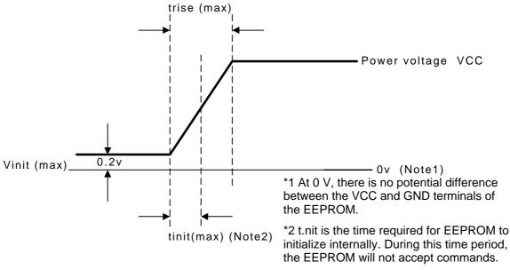
Fig. 1 Activation of the Power Voltage
