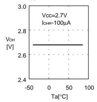
1.19 High level output voltage V<sub>OH</sub> – Ambient temperature Ta
