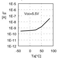
1.13 Input leakege current I<sub>LI</sub> – Ambient temprature Ta
