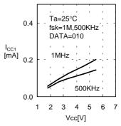
1.6 Current consumption (READ) I<sub>CC1</sub> - Clock frequency f<sub>SK</sub>
