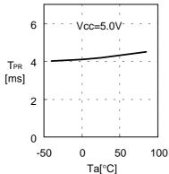
2.5 Program time T<sub>PR</sub> -Ambient temperature Ta
