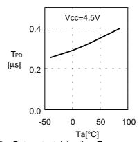
2.8 Data output delay time T<sub>PD</sub> -Ambient temperature Ta
