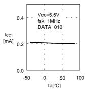
Current consumption (READ) I<sub>CC1</sub> – Ambient temperature Ta
