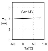
Data output delay time T<sub>PD</sub> -2.7 Ambient temperature Ta
