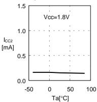
1.11 Stand by current consumption I<sub>SB</sub> – Ambient temperature Ta
