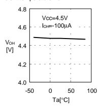
1.17 High level output voltage  $V_{\text{OH}}$  – Ambient temperature Ta
