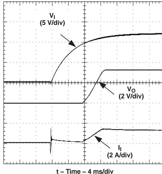
Figure 12. Power-Up Waveforms
