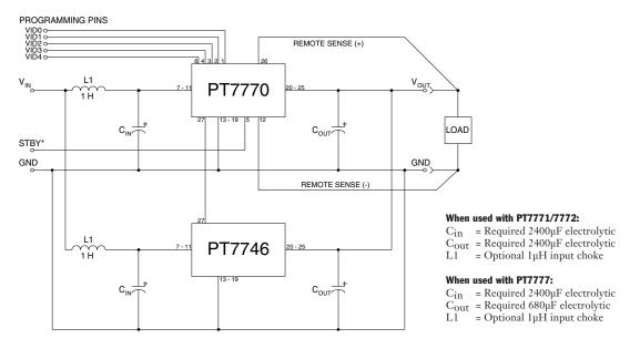
Output Capacitors: When used with a PT7771 or PT7772, the PT7746 requires a minimum ouput capacitance of 2400µE. When used with a PT7777, the PT7746 requires a minimum ouput capacitance of 680µE for proper operation. Do not use Oscon type capacitors. The maximum allowable output capacitance is 30,000µE.
