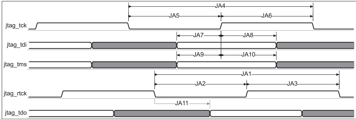
Figure 6-73. JTAG Interface Timing – Adaptive Clock Mode
