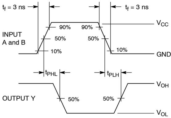
Figure 3. Switching Waveform
