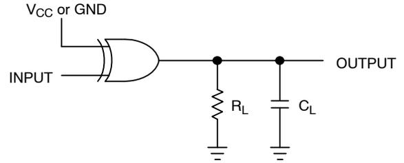
A 1-MHz square input wave is recommended for propagation delay tests.
