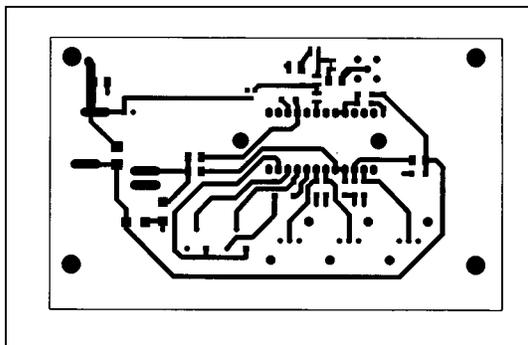
Figure 4. MAX445 EV Kit PC Board Layout—Component Side
