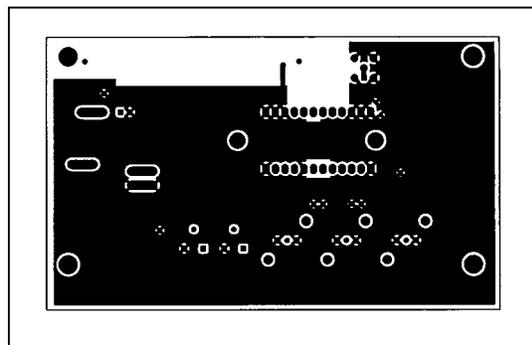
Figure 5. MAX445 EV Kit PC Board Layout—Solder Side
