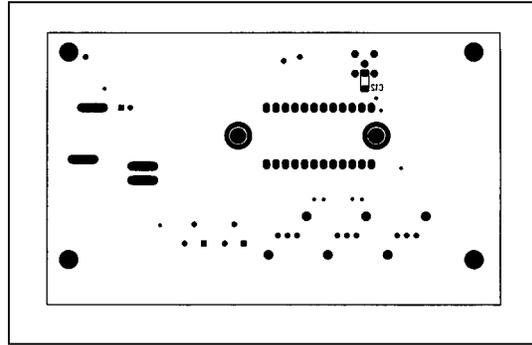
Figure 3. MAX445 EV Kit Component Placement Guide—Solder Side
