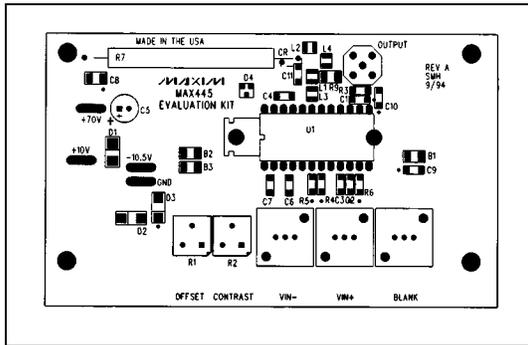
Figure 2. MAX445 EV Kit Component Placement Guide—Component Side
