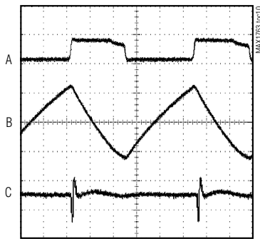
LIGHT-LOAD SWITCHING WAVEFORMS
