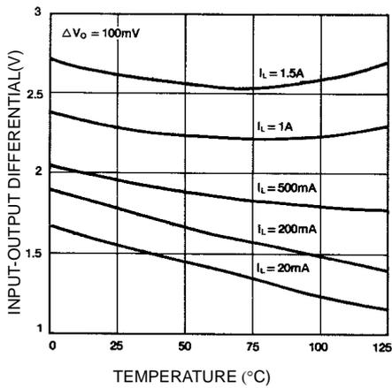
Figure 3. Dropout Voltage
