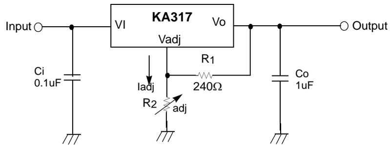
$$V_O = 1.25V (1+R_2/R_1)+I_{adj}R_2$$
