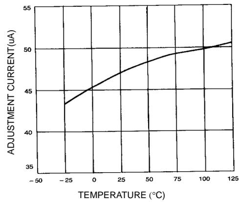
Figure 2. Adjustment Current
