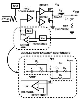
FIGURE 5. VOLTAGE-MODE BUCK CONVERTER COMPENSATION DESIGN
