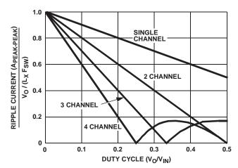
FIGURE 13. RIPPLE CURRENT vs DUTY CYCLE
