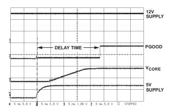
FIGURE 5. SUPPLY POWERED BY ATX SUPPLY
