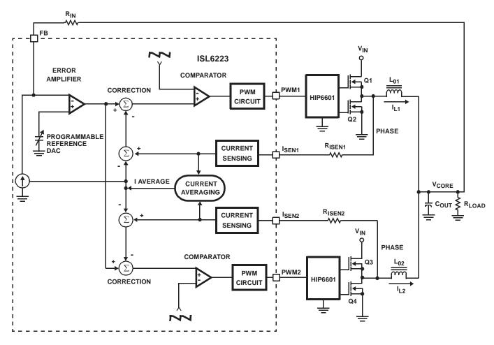
FIGURE 1. SIMPLIFIED BLOCK DIAGRAM OF THE ISL6223 VOLTAGE AND CURRENT CONTROL LOOPS FOR A TWO POWER CHANNEL REGULATOR
