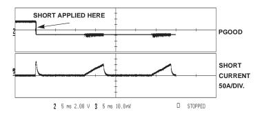
FIGURE 6. SHORT APPLIED TO SUPPLY AFTER POWER-UP
