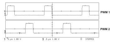
FIGURE 2. TWO PHASE PWM OUTPUT AT 500kHz
