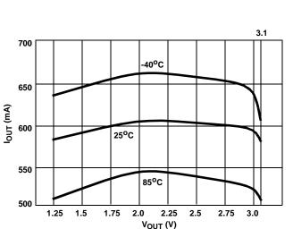
FIGURE 4. CURRENT REGULATION vs V<sub>OUT</sub> (VIN = 3.3V)
