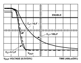
FIGURE 8. SLOW TURN-OFF vs  $C_{L.}R_{I}=8\Omega$
