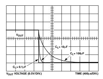
FIGURE 9. FAST TURN-OFF vs C<sub>LOAD</sub>S
