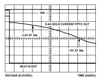
FIGURE 13. ISL6118 vs PPTC WITH EXTENDED 3.5 $\Omega$  LOAD
