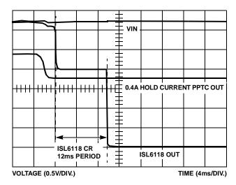
FIGURE 12. ISL6118 vs PPTC INTO  $3.5\Omega$  LOAD
