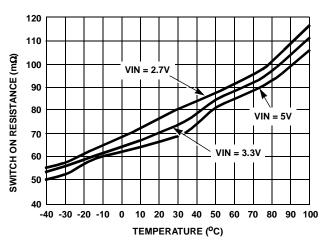
FIGURE 2. SWITCH ON RESISTANCE AT 0.4A
