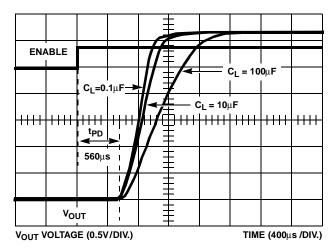
FIGURE 3.  $V_{OUT}$  SOFT START vs  $C_L$  and PROP DELAY,  $R_I$  =  $8\Omega$
