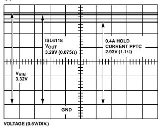
FIGURE 11. ISL6118 vs PPTC INTO 8.2Ω LOAD
