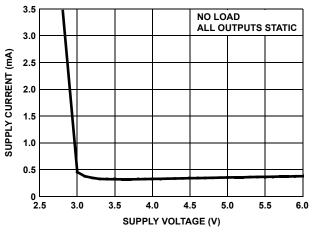
FIGURE 15. SUPPLY CURRENT vs SUPPLY VOLTAGE
