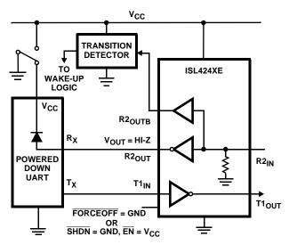
FIGURE 3. DISABLED RECEIVERS PREVENT POWER DRAIN
