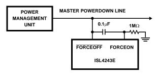
FIGURE 5. CIRCUIT TO PREVENT AUTO POWERDOWN FOR 100ms AFTER FORCED POWERUP
