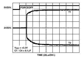
FIGURE 8. TRANSMITTER OUTPUTS WHEN EXITING POWERDOWN
