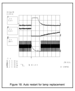
Recovery from such a fault condition is accomplished by cycling either the SD lead or the  $V_{CC}$  lead. When a lamp is removed, the SD lead goes high, the fault latch is reset, and the chip is held off in an unlatched state. Lamp replacement causes the SD lead to go low again, reinitiating the startup sequence. The fault latch can also be reset by the undervoltage lockout signal, if  $V_{CC}$  falls below the lower undervoltage threshold.
