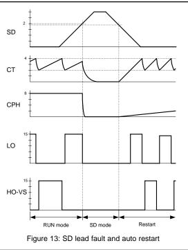
conditions a reset signal would restart the chip from the beginning of the control sequence, as shown in the timing diagram in Figure 13.
