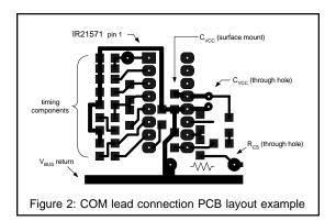
This connection technique prevents high current ground loops from interfering with the sensitive timing component operation, and allows the entire control circuit to reject common-mode noise due to output switching.
