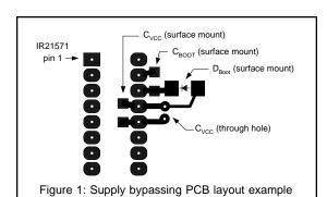
A rule of thumb for the value of this bypass capacitor is to keep its minimum value at least 2500 times the value of the total input capacitance (Ciss) of the power transistors being driven. This decoupling capacitor can be split between a higher valued electrolytic type and a lower valued ceramic type connected in parallel, although a good quality electrolytic (e.g.,  $10\mu F$ ) placed immediately adjacent to the Vcc and COM terminals will work well.
