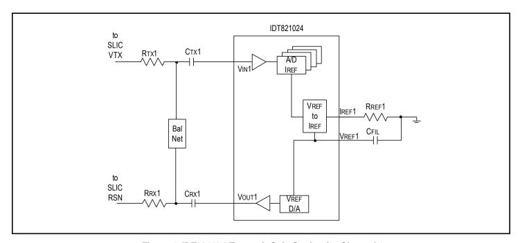
Figure 1. IDT821024 Transmit Gain Setting for Channel 1
