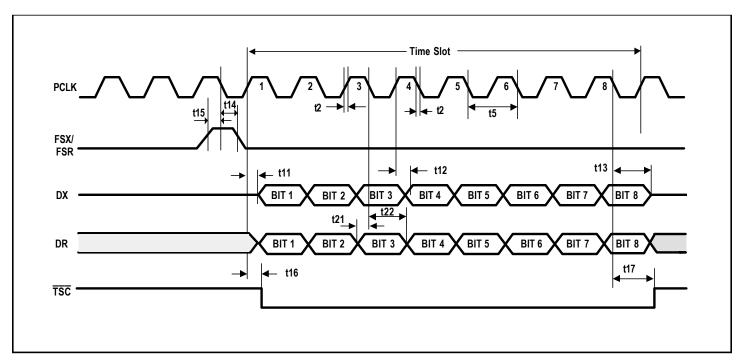
Figure 3. PCM Interface Timing for Short Frame Mode
