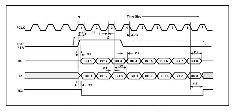
Figure 4. PCM Interface Timing for Long Frame Mode
