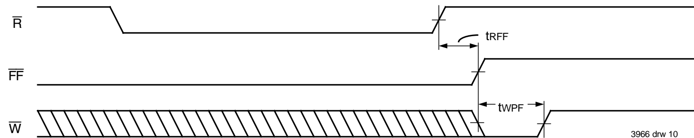
Figure 8. Minimum Timing for a Full Flag Coincident Write Pulse
